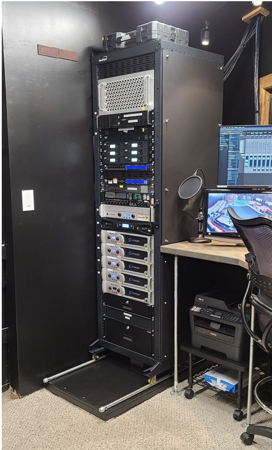
New sound rack on wheels to allow better access to rear for maintenance. Printer on cart below desk frees desk space while still keeping nearby.
